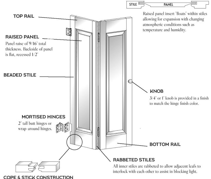
All panels are joined with cope & stick type construction for greater strength.
